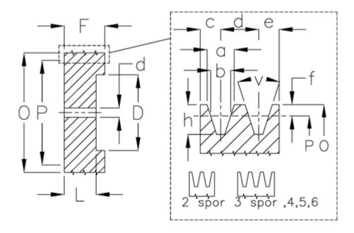
$\begin{array}{lll} D & = 93 \\ d & = 20 \\ F & = 136.0 \\ L & = 96 \\ Number of ribs = 5 \\ O & = 159.6 \\ P & = 150 \\ Type & = C \\ \end{array}$
